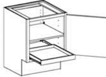
Passport Base Single Door w/Full Width Tray (ABFH_•FWT) Available sizes: Width: 12, 15, 18, 21, 24, 27 Depth: 24 Height: 32½
